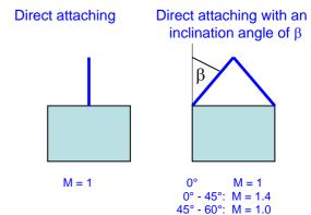
**Note:** never select an angle of inclination  $\beta$  greater than 60°
