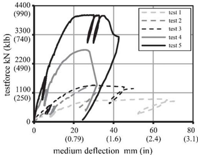
Figure 7 — Load deflection curves of the slabs
