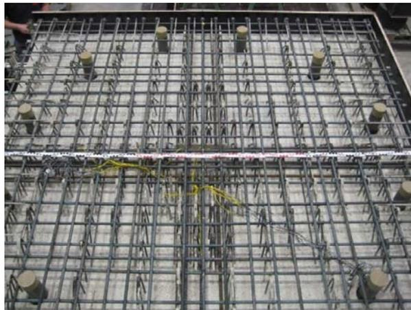
Figure 6 — Test specimen no. 3 with FDB II 21/3 before concreting the top layer
