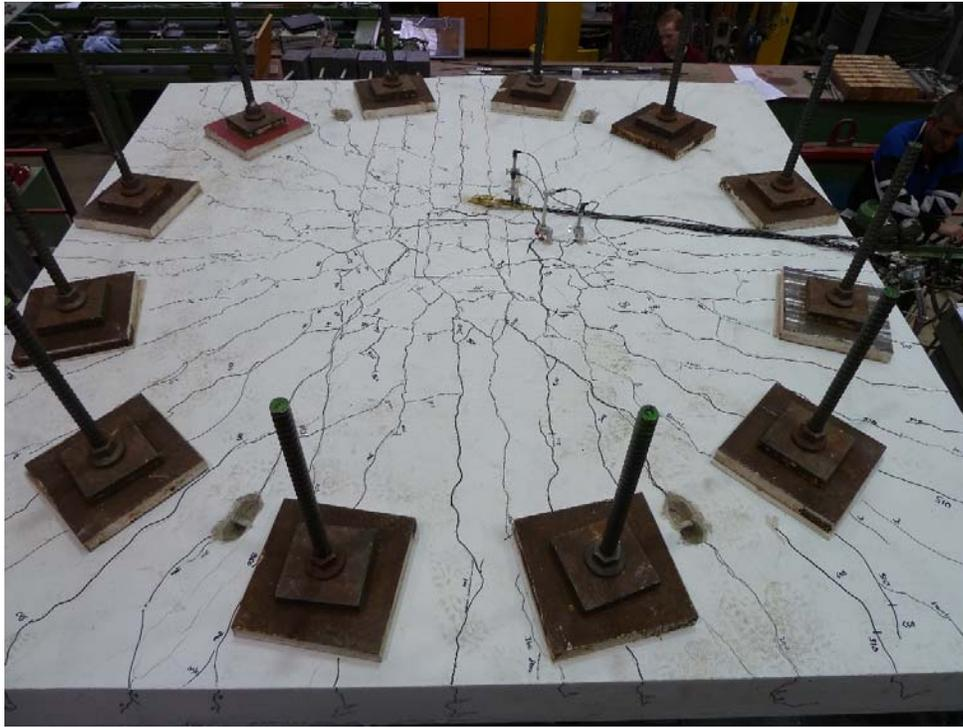
Figure 8 — Crack pattern of the upper surface of test no. 3 in Table 1
