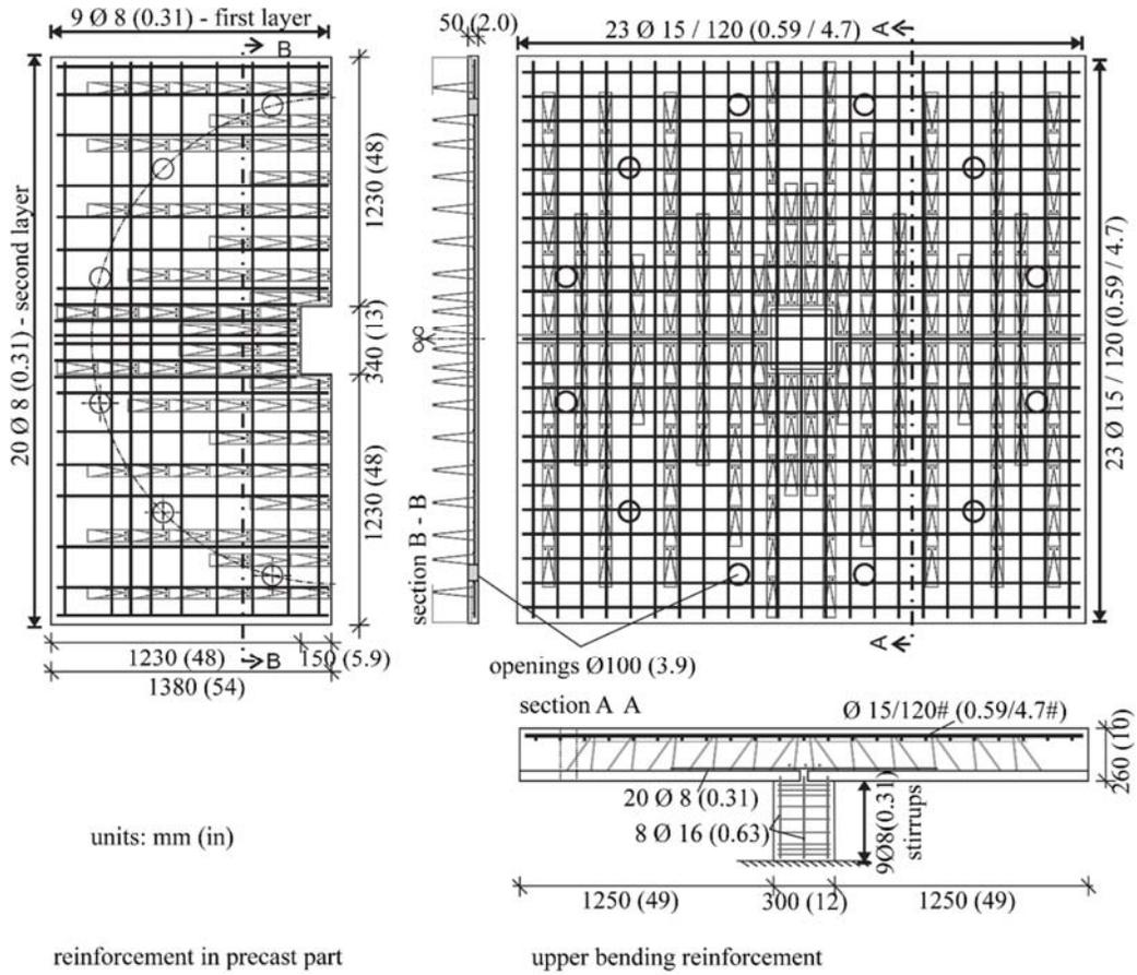
Figure 5 — Test specimen with Filigran Punching Shear Reinforcement (example FDB II 21/3)
