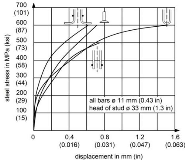
Figure 2 — Steel stress slip curves for different anchorages according to Furche (2007)
