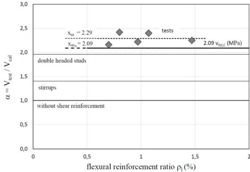
Figure 11 — Evaluation of the increasing factors according to DIN EN 1992-1-1/NA with eq. (1)
