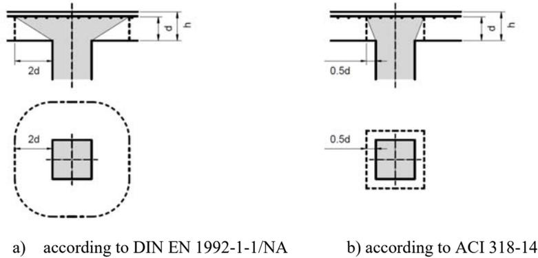
Figure 10 — Different control perimeter for proving the punching shear resistance
