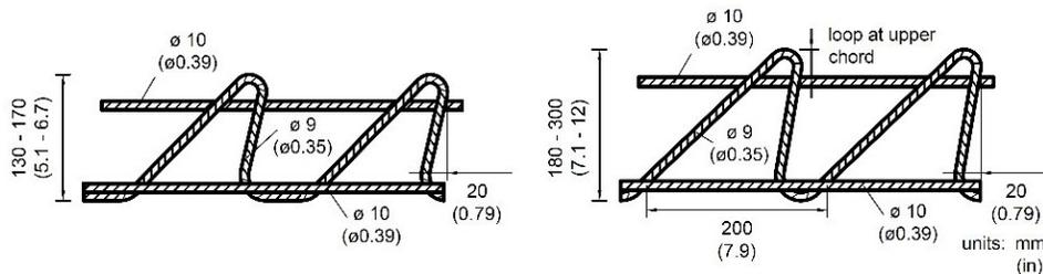
Figure 3 — Filigran Punching Shear Reinforcement according to ETA-13/0521 (2013)
