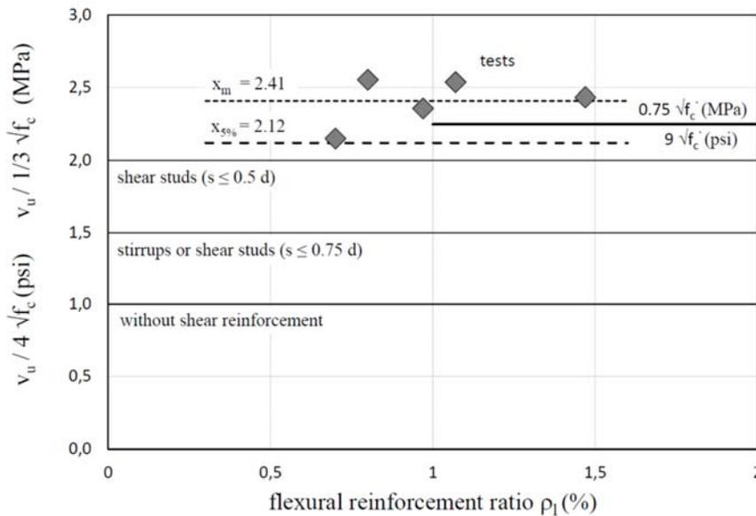
Figure 12 — Evaluation of the maximum test loads according to ACI 318-14 with eq. (3)
