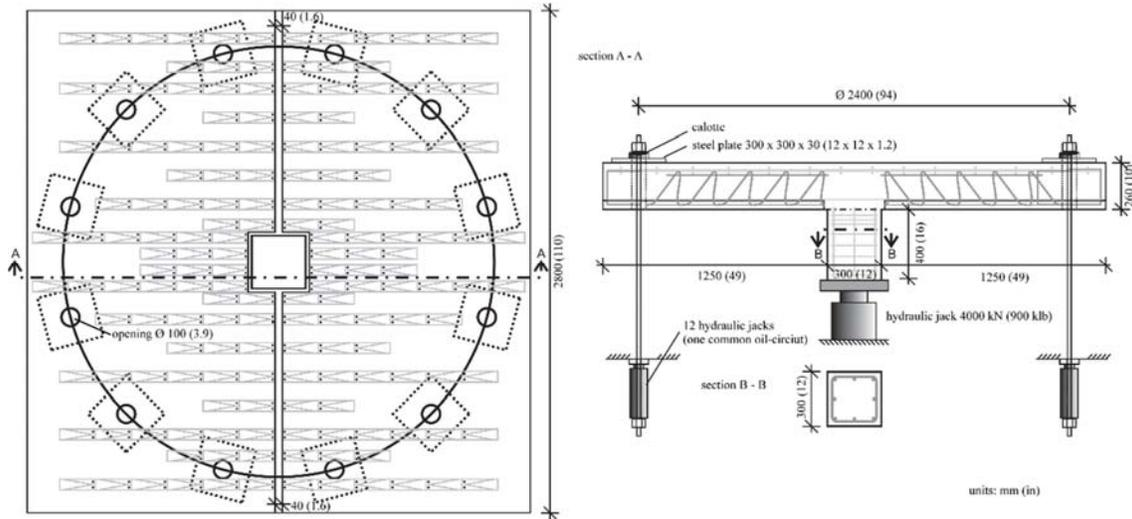
Figure 4 — Test arrangement
