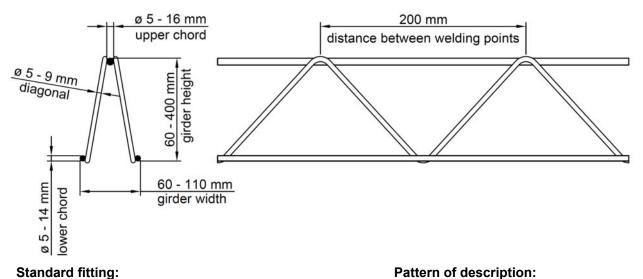
Normal ductile (A) reinforcing steel B500A Yield strength  $R_e^{(1)} \ge 500 \text{ MPa} (N/mm^2)$ Ratio of tensile strength / yield stress  $R_m$  /  $R_e^{-1} \ge 1.05$ Elongation at tensile strength  $A_{gt} \ge 2.5\%$ <sup>1)</sup> or 0.2% proof strength respectively
